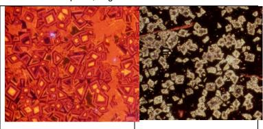
CL image of zoned dolomite crystal fabric suggests that dolomitisation involves flux of redox sensitive elements. most likely Mn and Fe) as well as magnesium. Field of view ~1mm.
