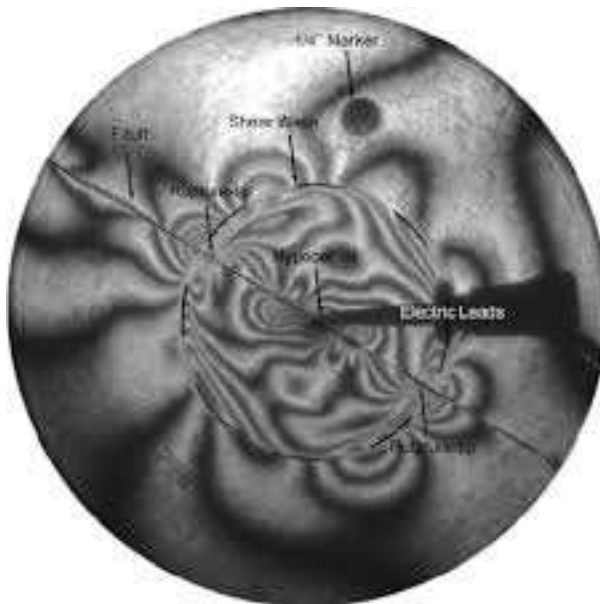
Figure 1. Earthquakes in the laboratory captured using high-speed photography. The fringes shown illustrate the strain field around the propagating rupture in a photo-elastic material.
